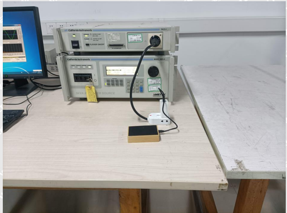
Harmonic/Flicker Test View
