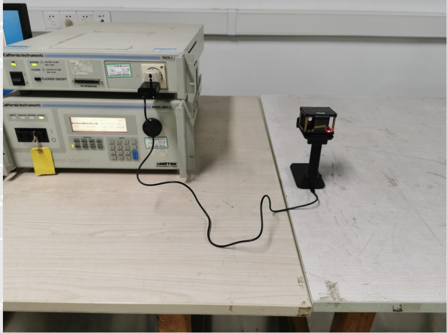
Harmonic/Flicker Test View
