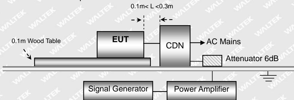
For Signal or Telecommunication Ports:
