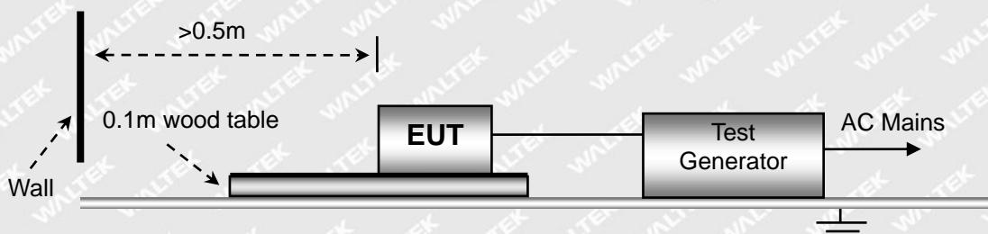
For Signal or Telecommunication Ports:
