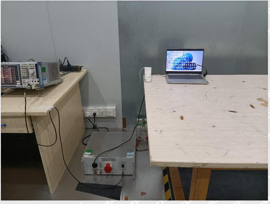
A photograph showing the conducted emission test setup. On the left, a wooden bench holds a signal generator and a power source unit connected by various cables. To the right, a laptop sits on a light-colored wooden table, connected to a device on the bench. A metal shelving unit is visible in the background. |
