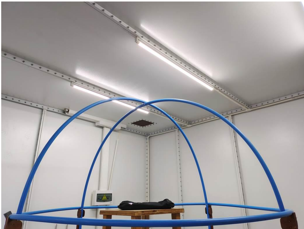
EN IEC 55015 RADIATED ELECTROMAGNETIC DISTURBANCE TEST
