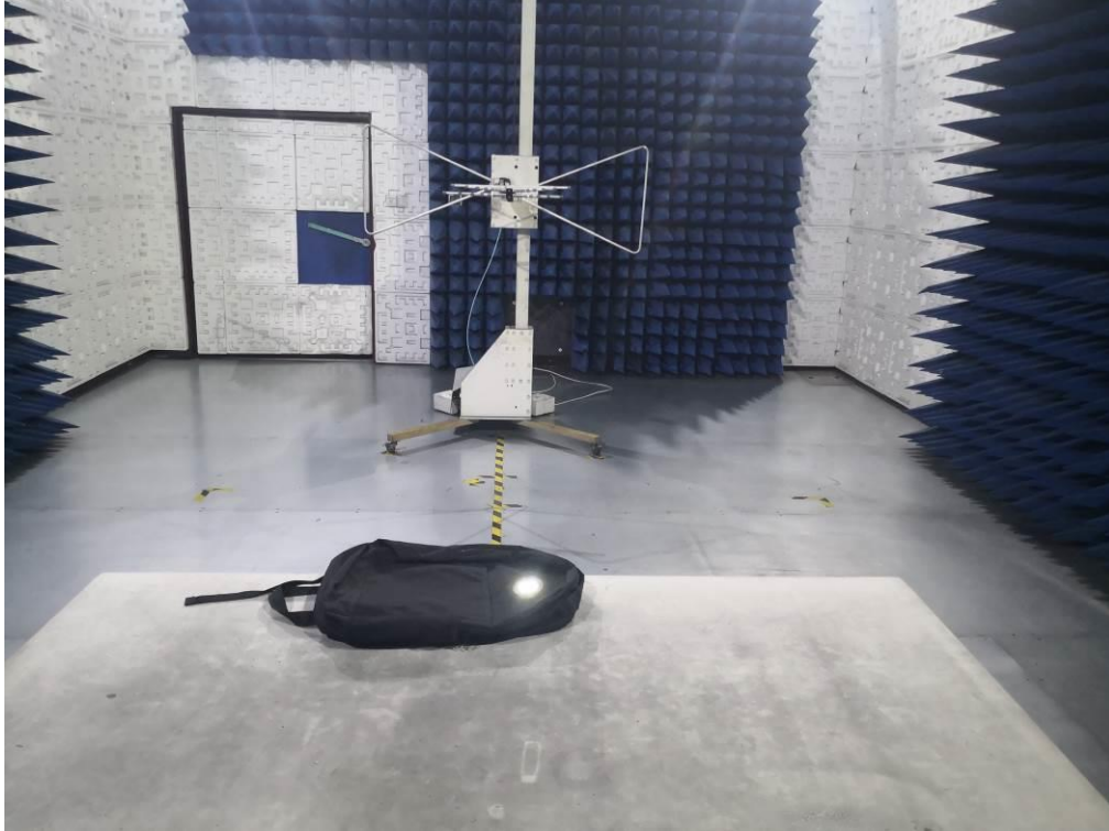
EN IEC 55015 RADIATED ELECTROMAGNETIC DISTURBANCE TEST
