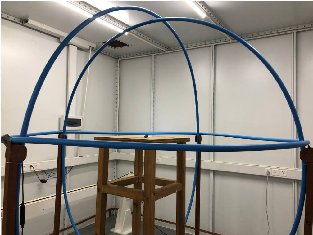
EN 61000-4-3 RS IMMUNITY TEST SETUP
