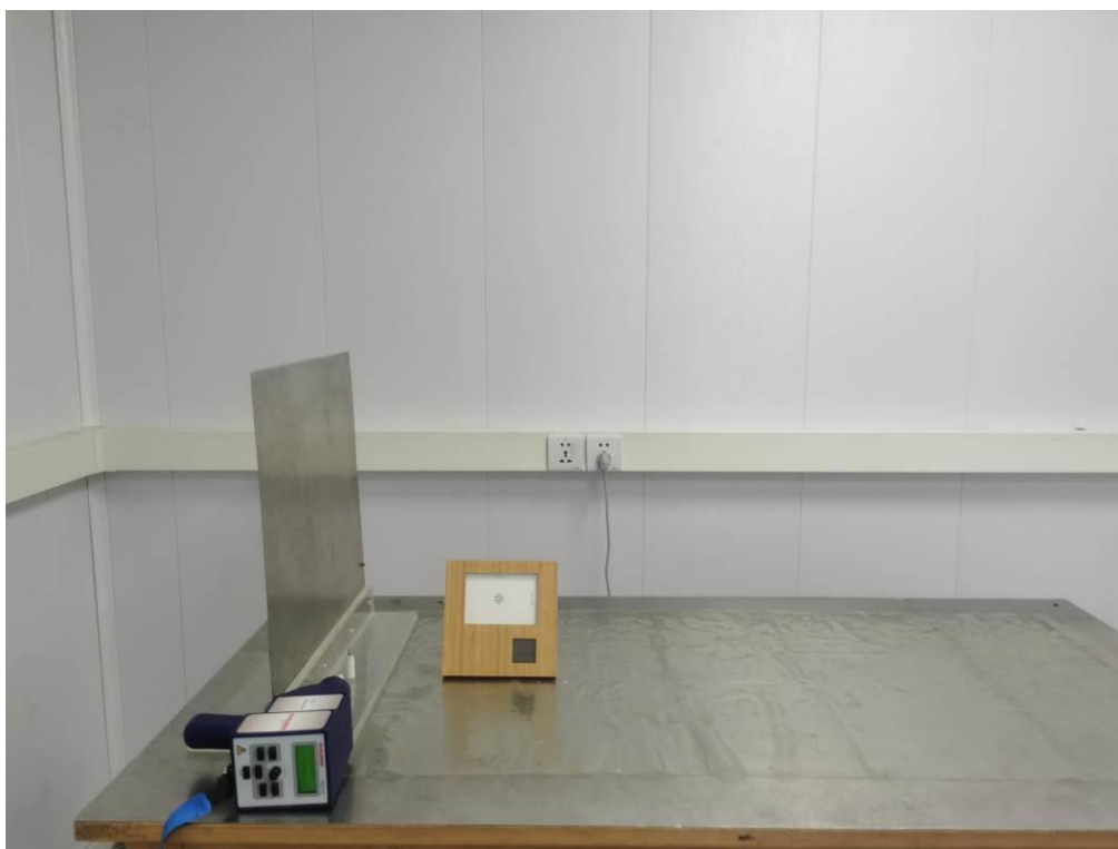
Test Setup Photo of Electrostatic Discharge Test
